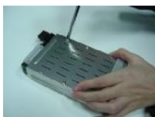
Step 4 Loosen all screws on the Cartridge
